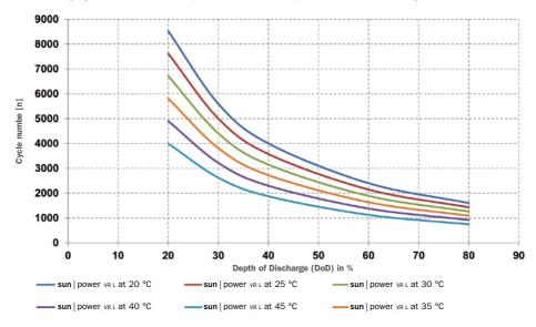
Fig. 7-10: Endurance in cycles of sun | power VR L (OPzV solar.power) depending on DoD and temperature
