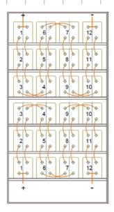
In general, connect the batteries using the shortest possible cables. Normally, cells are connected in series with alternating polarity, resulting in the shortest possible connector length.
