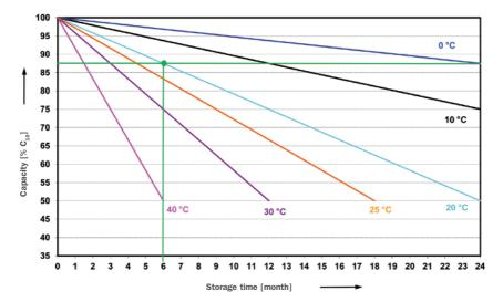
Fig. 4-1: Available Capacity vs. storage time
