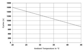
Fig. 7-9: Endurance in cycles of sun | power VR L (OPzV solar.power) as a function of ambient temperature
