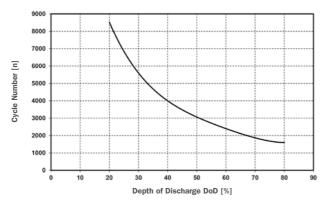
Fig. 7-8: Endurance in cycles of sun | power vR L (OPzV solar.power) as a function of DoD (at 20°C)
