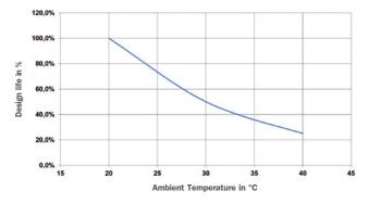
Fig. 7–7: Design life of  $un \mid$  power vRL (OPzV solar.power) cell as a function of ambient temperature (standby application in float charge operation with 2.25 V/cell)
