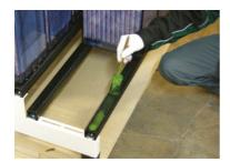
Fig. 5-13: Greased support profiles
