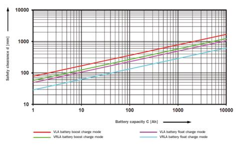
Fig. 5-1: Safety distance based on battery capacity (Source HOPPECKE)
