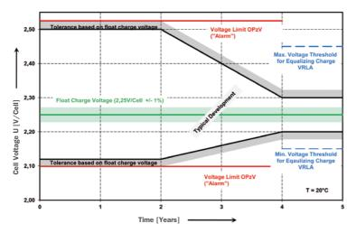
Fig. 6-4: Trend of float charge voltage over service life of gel batteries.
